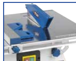
Workbench with fence and accessory for 45° cuts
